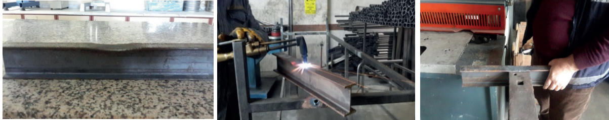
Figure 5. Heat Treating and Correction of Locally Deformed Specimen
