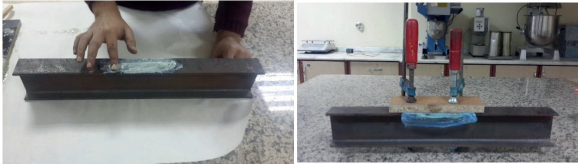
Figure 6. Applying Epoxy and CFRP and Clamping to the Specimen
